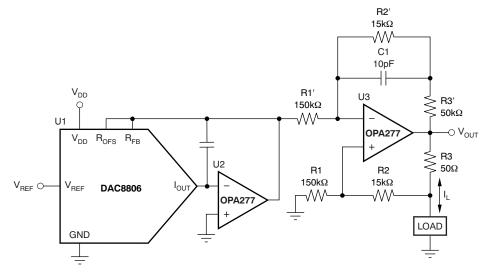
Figure 43. Programmable Bidirectional Current Source Circuit
