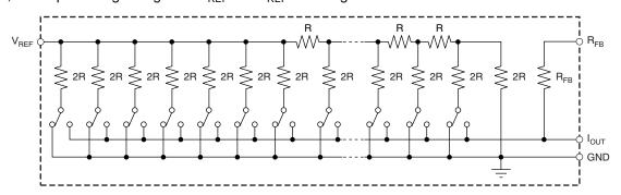
Figure 38. Equivalent R-2R DAC Circuit
