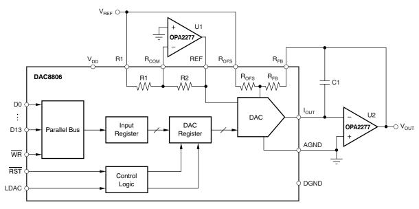
Figure 42. Bipolar Output Circuit
