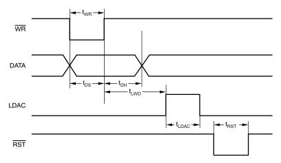
Figure 40. DAC8806 Timing Diagram
