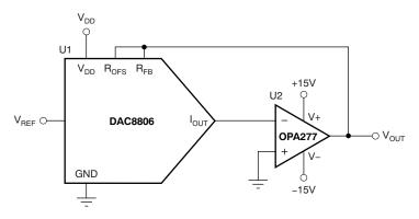
Figure 39. Voltage Output Configuration
