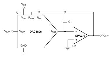
Figure 41. Gain Peaking Prevention Circuit with Compensation Capacitor
