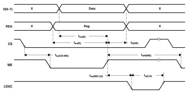
Figure 1. Timing Diagram
