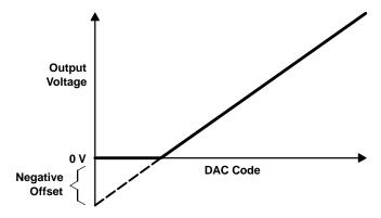
Figure 12. Effect of Negative Offset (Single Supply)
