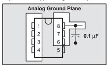
Figure 16. Power-Supply Bypassing
