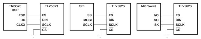
Figure 16. Three-Wire Interface
