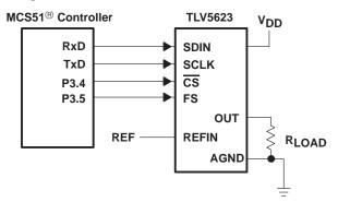
Figure 18. TLV5623 to MCS51<sup>®</sup> Controller Interface
