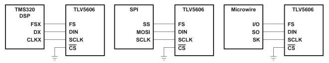
Figure 16. Three-Wire Interface
