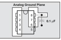
Figure 20. Power-Supply Bypassing
