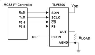
Figure 18. TLV5606 to MCS51<sup>®</sup> Controller Interface
