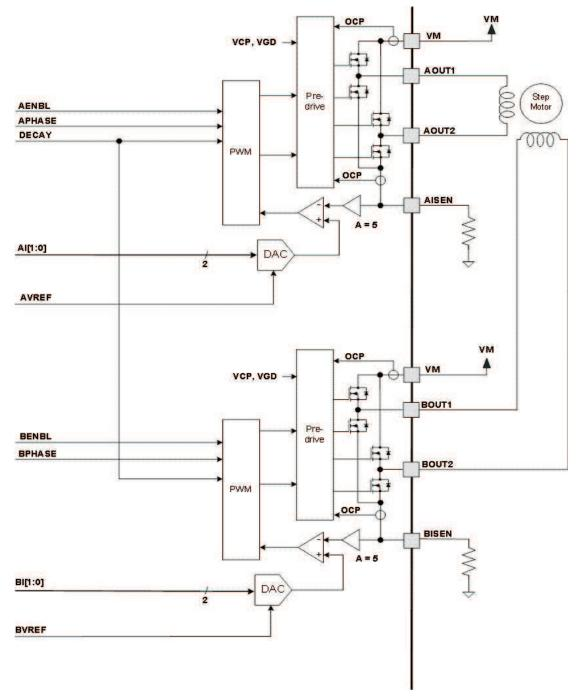
Figure 5. Motor Control Circuitry
