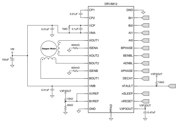
Figure 7. Typical Application Schematic
