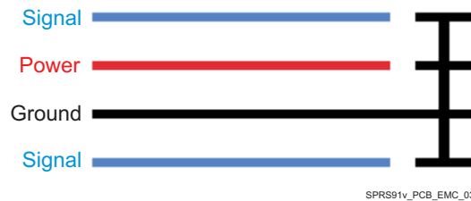
图 7-13. Guard Ring Routing
