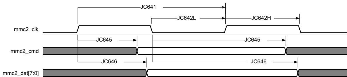
Figure 7-78. MMC/SD/SDIO in - High Speed JC64 - Transmitter Mode
