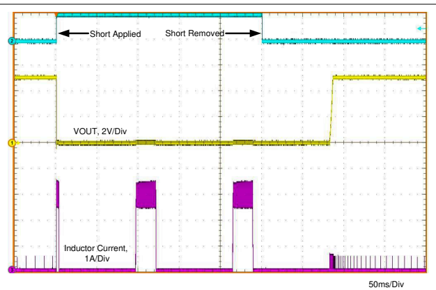
图 7-6. Short-Circuit Transient and Recovery
