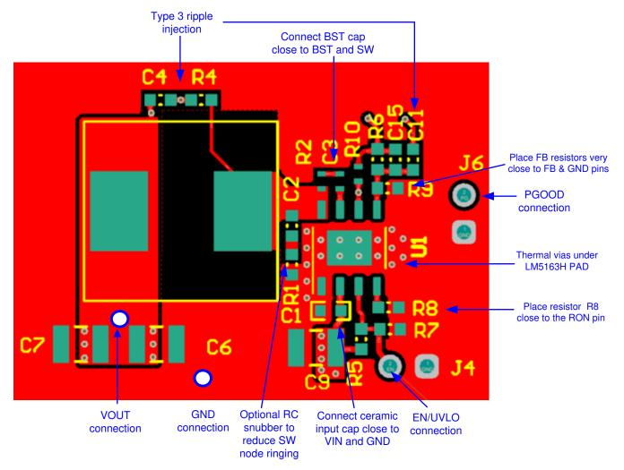
图 30. LM5163H-Q1 Single-Sided PCB Layout Example
