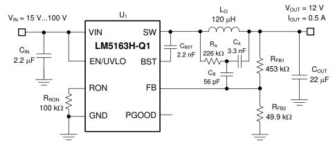
图 12. Typical Application  $V_{IN(nom)} = 48 \text{ V}$ ,  $V_{OUT} = 12 \text{ V}$ ,  $I_{OUT(max)} = 0.5 \text{ A}$ ,  $F_{SW(nom)} = 300 \text{ kHz}$
