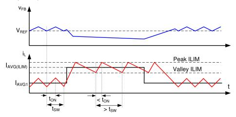
图 11. Current Limit Timing Diagram
