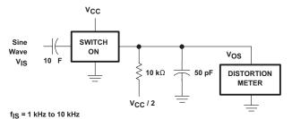
Figure 2. Sine-Wave Distortion Test Circuit
