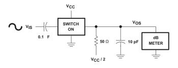
Figure 1. Frequency-Response Test Circuit
