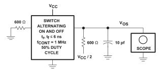
Figure 3. Control-to-Switch Feedthrough Noise Test Circuit
