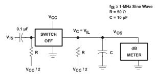
Figure 4. Switch OFF Signal Feedthrough Test Circuit
