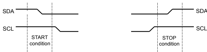
Figure 21-3. START and STOP Conditions
