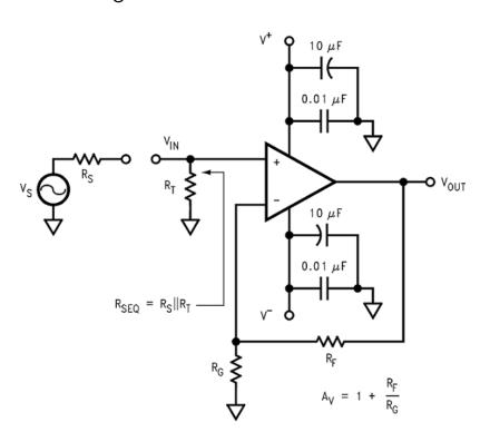
Figure 32. Typical Non-Inverting Application
