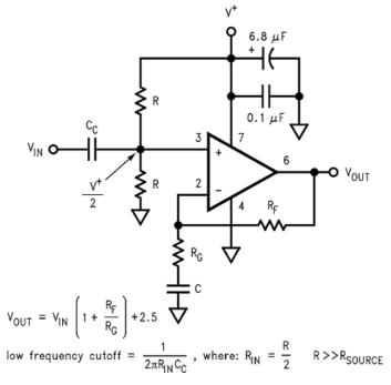
Figure 35. AC Coupled Non-Inverting
