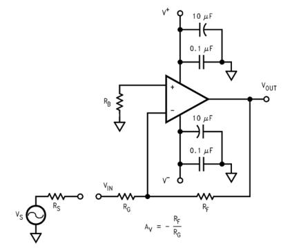
Figure 33. Typical Inverting Application
