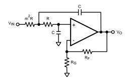
Figure 1. Sallen Key Low Pass Filter with Equal C Value
