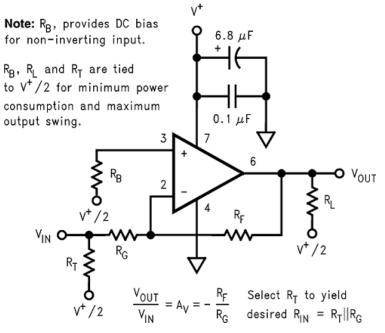
Figure 34. Single Supply Inverting
