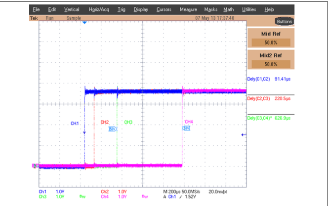
Figure 26. Power up with different tD settings
