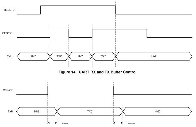
Figure 15. CFG/OE to TXH Timing
