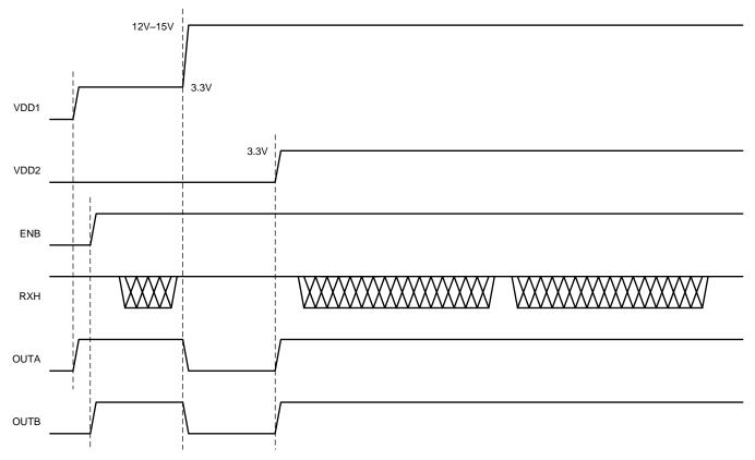
Figure 9. Typical Startup in Normal Mode
