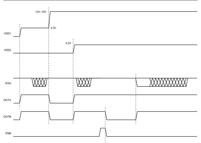
Figure 10. Typical Startup Timing for Control Mode
