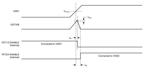
Figure 13. VDD Switch-over at VDD1 Rising Above  $V_{HVLO}$
