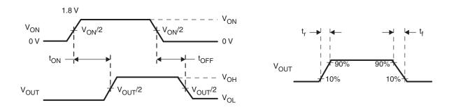
A.  $t_{rise}$  and  $t_{fall}$  of the control signal is 100 ns.
