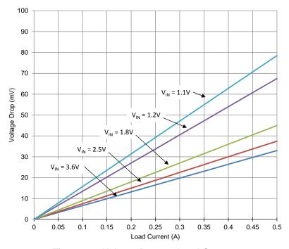
Figure 29. Voltage Drop vs Load Current
