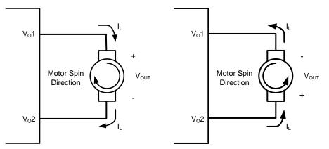
Figure 19. Voltage Polarity and Motor Direction
