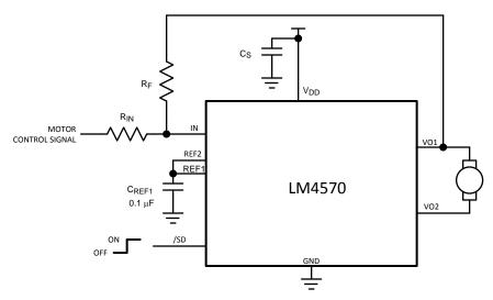
Figure 1. Typical Motor Driver Application Circuit
