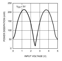
Figure 20. Power Dissipation vs. Input Voltage
