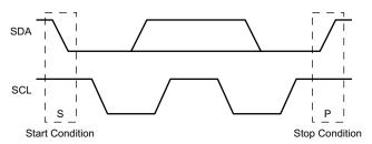
图 8-23. I<sup>2</sup>C Definition of Start and Stop Conditions
