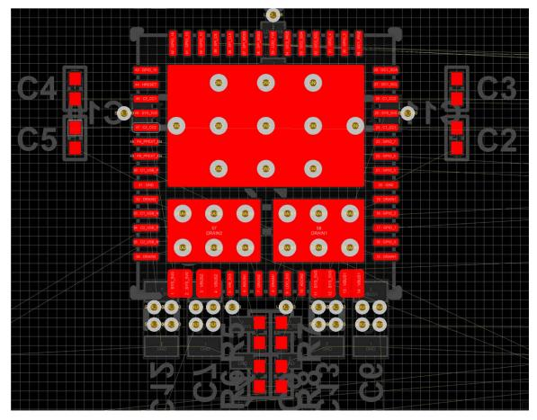
图 11-12. CC and ADCIN1/2 Component Placements
