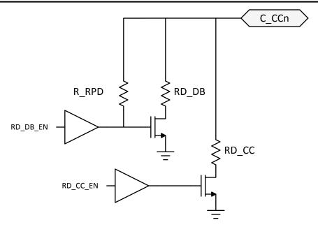
图 8-16. Dead Battery Pull-Down Resistor
