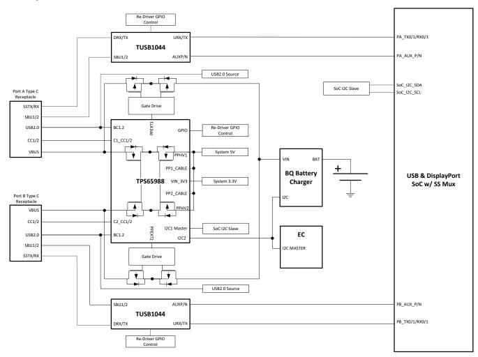
图 9-9. TPS65988 and SoC I2C with Re-Driver GPIO
