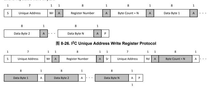
图 8-27. I<sup>2</sup>C Unique Address Read Register Protocol
