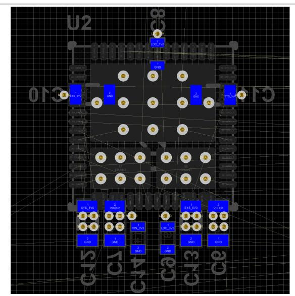
图 11-11. System Capacitors Placement Bottom Layer
