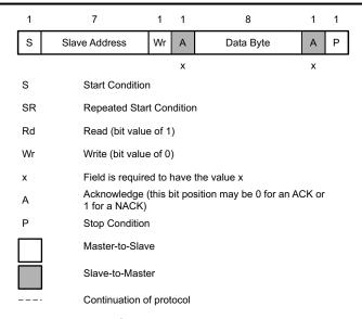
图 8-28. I<sup>2</sup>C Read/Write Protocol Key
