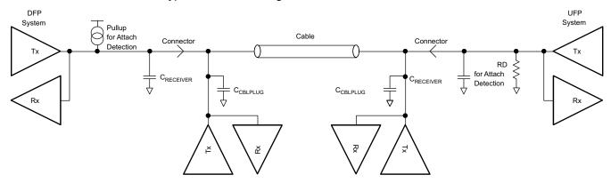
图 8-8. Example USB-PD Multi-Drop Configuration
