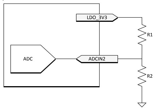
图 8-29. I<sup>2</sup>C Address Divider
