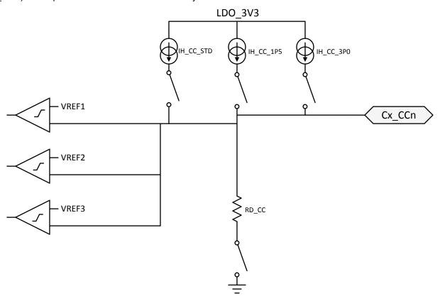
图 8-14. Plug and Orientation Detection Block
