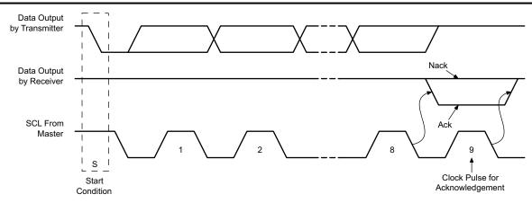
图 8-25. I<sup>2</sup>C Acknowledgment
