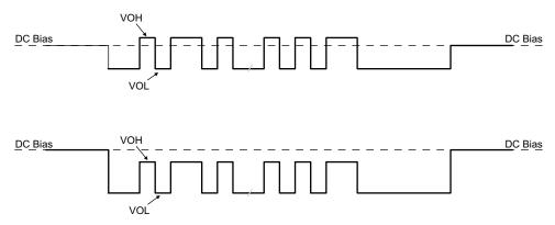
图 8-6. TX Driver Transmission with DC Bias
