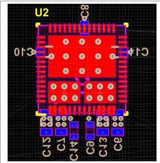
图 11-9. System Capacitors Placement Top/Bottom Layer
