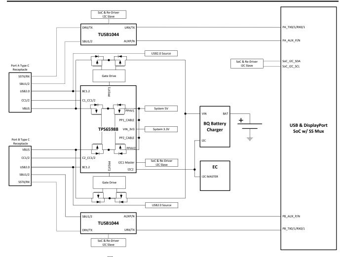
图 9-10. TPS65988 and SoC & Redriver I2C
