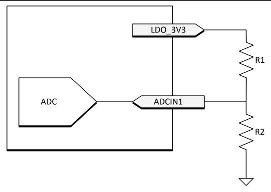
图 8-17. ADCIN1 Resistor Divider
