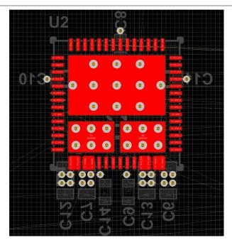
图 11-10. System Capacitors Placement Top Layer
