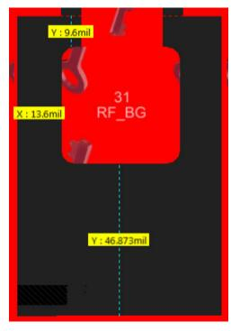
图 10-5. Top Layer Copper Pull Back on RF Pads
