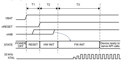
图 8-6. First-Time Power-Up and Reset Removal Timing Diagram
