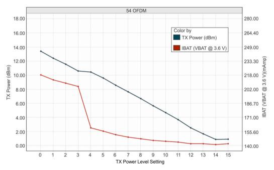
图 8-3. TX Power and IBAT vs TX Power Level Settings (54 OFDM)
