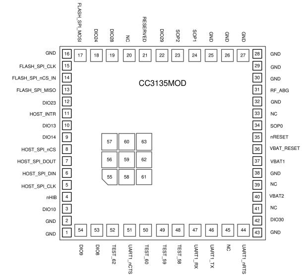
图 7-1 shows the approximate location of pins on the module.
