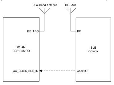
图 10-1. Dual-Antenna Coexistence Mode Block Diagram
