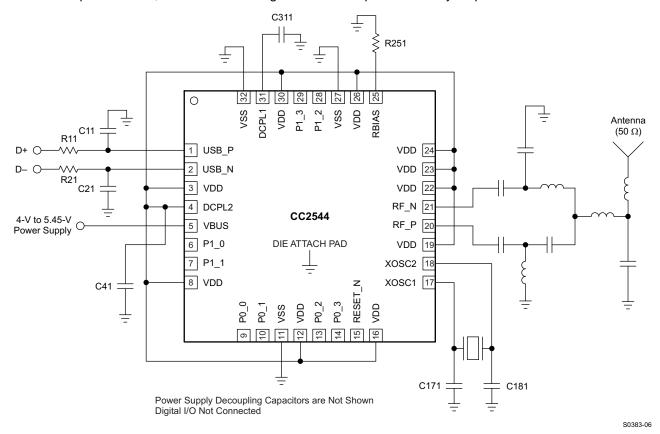
Figure 19. CC2544 Application Circuit
