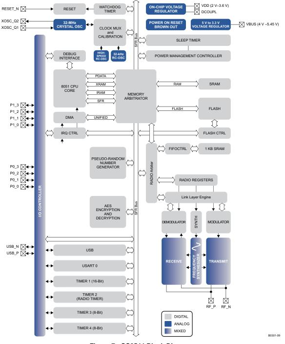
Figure 7. CC2544 Block Diagram
