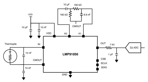
Figure 26. Typical NDIR Sensing Application Circuit
