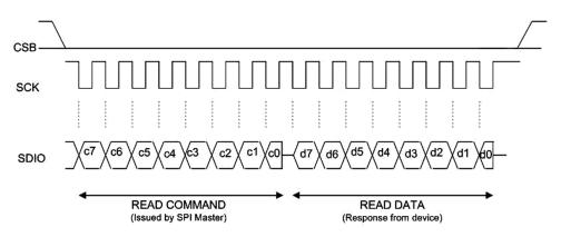
Note: Read command is issued by the SPI Master, who after issuing the c0 (LSBit of the command byte) bit should relinquish the data line (high-Z) after meeting the hold timing(10ns) and stop SCK idling high.
