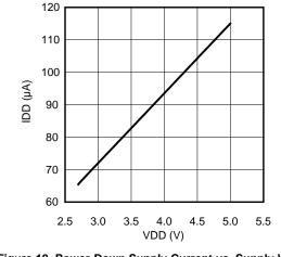
Figure 19. Power-Down Supply Current vs. Supply Voltage
