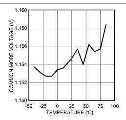
Figure 15. Common-Mode Voltage vs. Temperature
