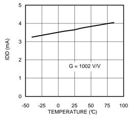
Figure 17. Supply Current vs. Temperature
