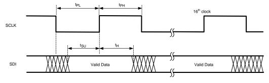
Figure 2. SPI Set-Up Hold Time
