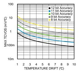
Figure 22. System Accuracy vs. TCVOS and Temperature Drift
