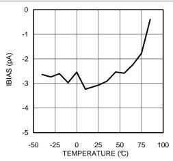
Figure 16. Input Bias Current vs. Temperature
