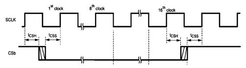
Figure 1. SPI Timing Diagram
