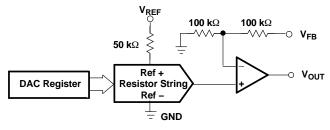
Figure 43. Typical DAC Architecture
