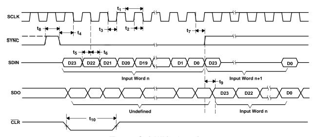
Figure 1. Serial Write Operation
