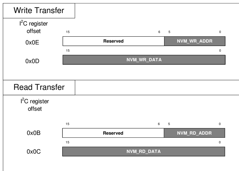
Figure 28. EEPROM Direct Access Using I 2 C
