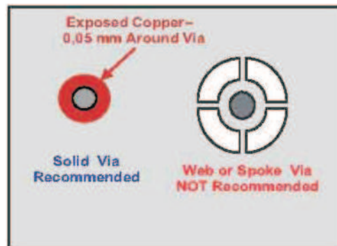
Figure 27. Thermal Via Connection at the Bottom Layer
