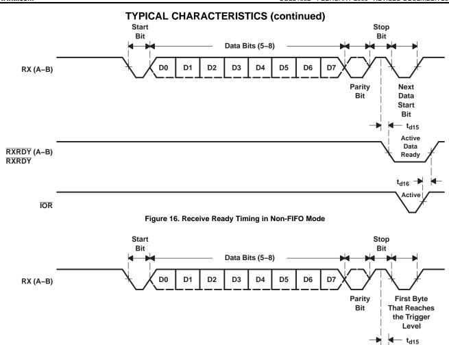
Figure 17. Receive Timing in FIFO Mode
