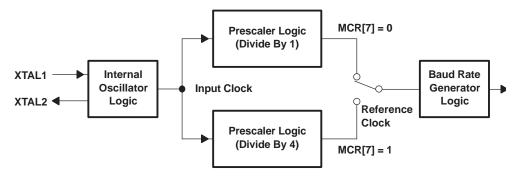
Figure 9. Prescaler and Baud Rate Generator Block Diagram
