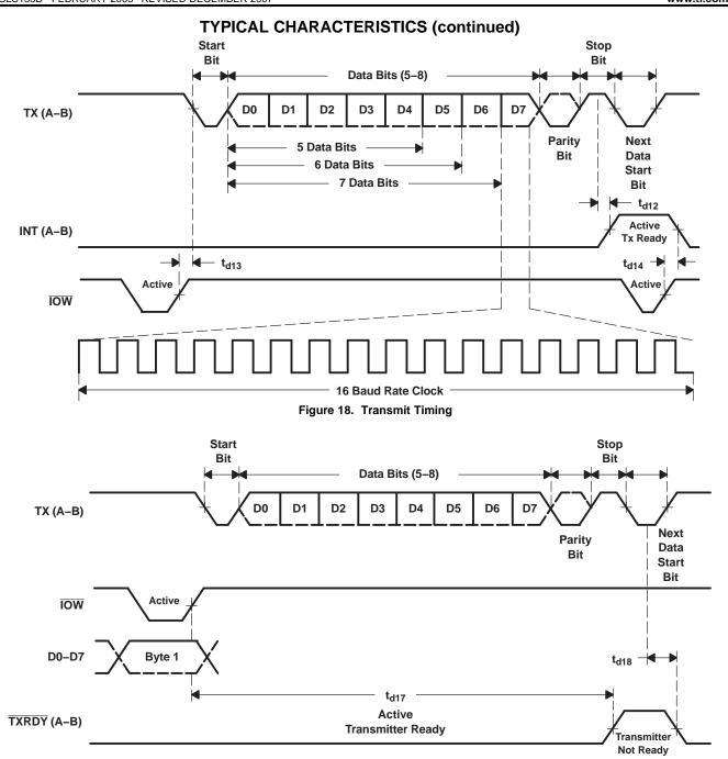
Figure 19. Transmit Ready Timing in Non-FIFO Mode
