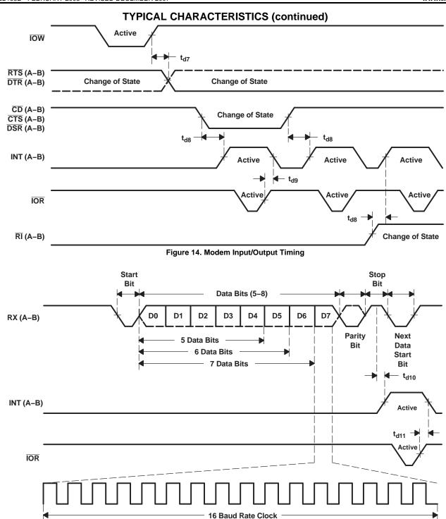
Figure 15. Receive Timing
