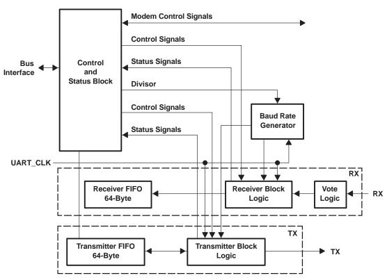
A. The vote logic determines whether the RX data is a logic 1 or 0. It takes three samples of the RX line and uses a majority vote to determine the logic level received. The vote logic operates on all bits received.
