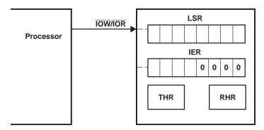
Figure 6. FIFO Polled Mode Operation
