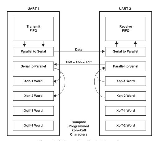
Figure 4. Software Flow Control Example
