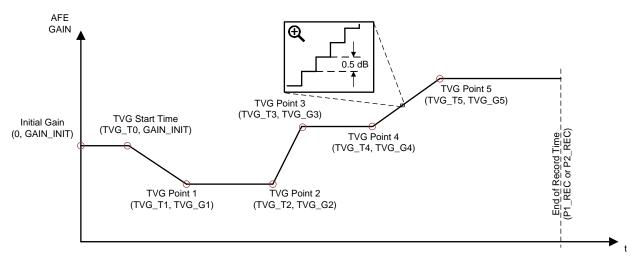
图 6. Time-Varying Gain Assignment Example
