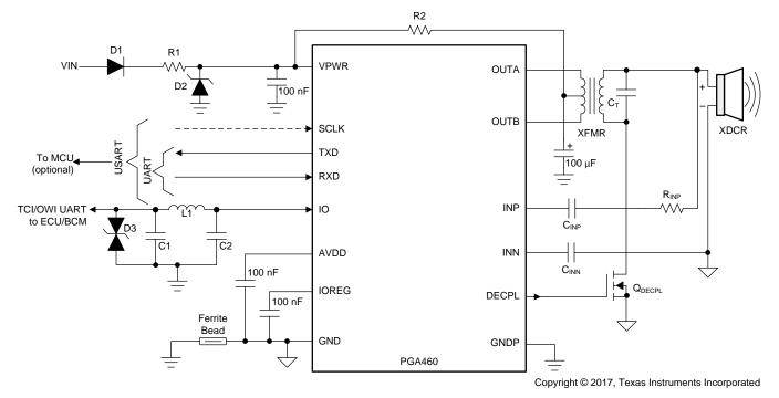
图 136. Transformer-Driven Method Schematic
