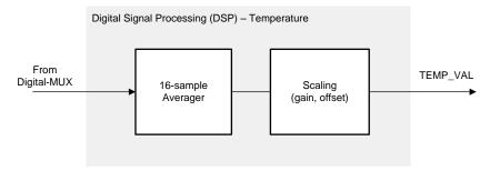
图 41. Temperature-Sensor Signal Path
