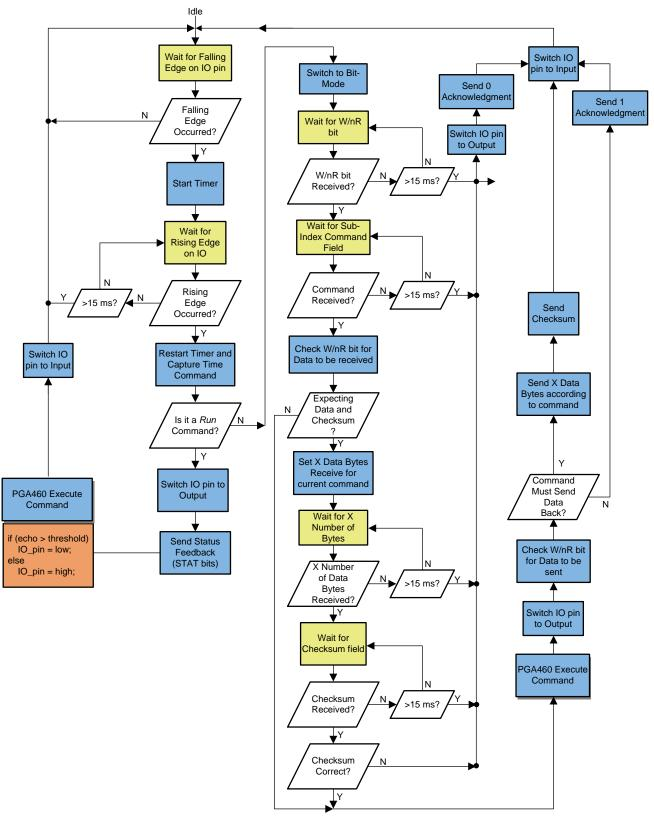
图 44. Time-Command Interface Communication Flow Chart
