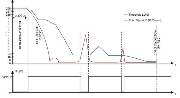
图 15. IO-Pin Object-Detection Signaling With Burst/Listen Time Command
