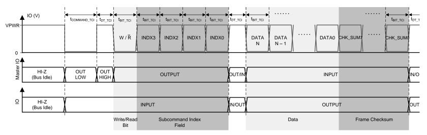
图 18. Time-Command Interface CONFIGURATION/STATUS Command—Read
