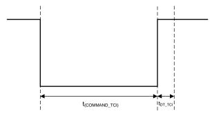
图 12. Time-Command Interface Command Timing
