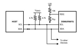
Figure 22. Serial Control Bus Connection
