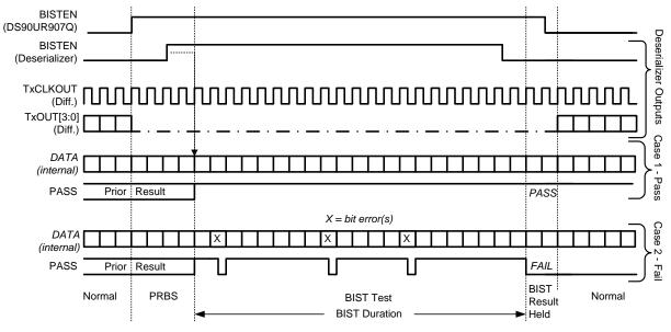
Figure 21. BIST Waveforms
