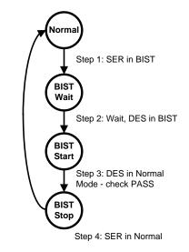
Figure 20. BIST Mode Flow Diagram
