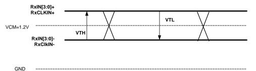
Figure 2. FPD-Link DC VTH/VTL Definition
