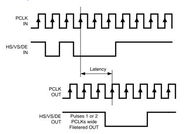
Figure 16. Video Control Signal Filter Wavefrom
