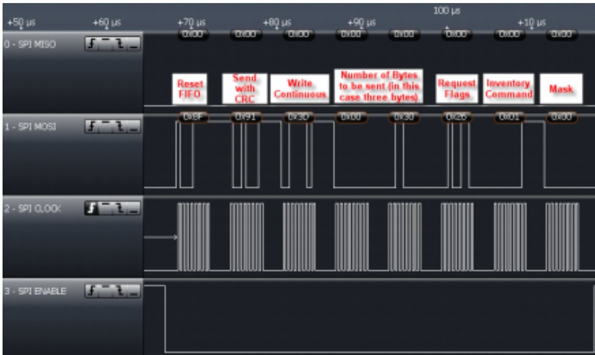
Figure 6-22. Inventory Command Sent From MCU to TRF7964A
