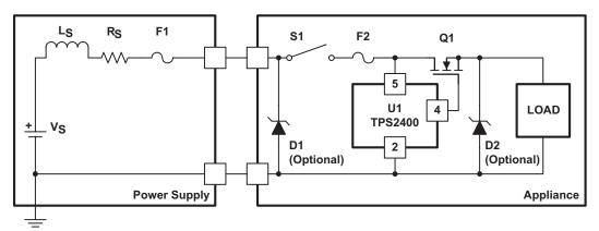
Figure 15. TPS2400 Application Block Diagram
