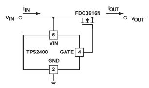
Figure 13. Application Diagram
