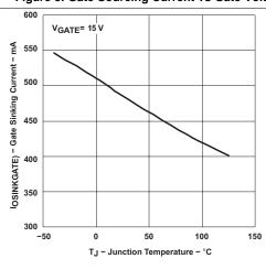
Figure 5. Gate Sinking Current vs Junction Temperature
