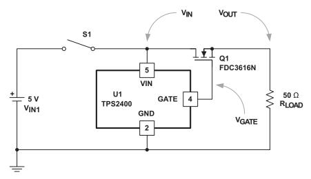
Figure 10. Output Turnon Response Test Circuit
