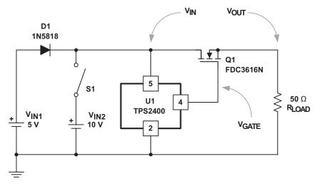
Figure 12. Output Turnoff Response Test Circuit
