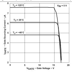
Figure 3. Gate Sourcing Current vs Gate Voltage
