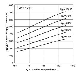
Figure 1. Input Supply current vs Junction Temperature
