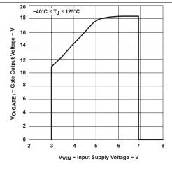
Figure 6. Gate Output Voltage vs Input Supply Voltage
