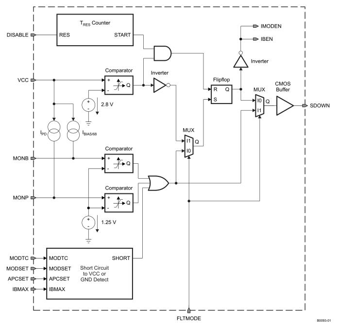
Figure 2. Functional Representation of the Fault Detection Circuitry
