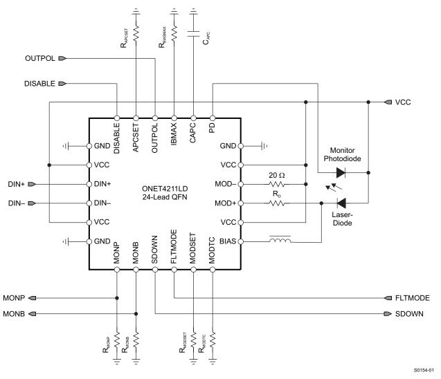
Figure 25. Basic Application Circuit With DC-Coupled Interface Between the ONET4211LD and the Laser Diode
