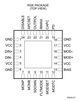
Figure 3. Pinout of the ONET4211LD in a 4-mm  $\times$  4-mm, 24-Lead QFN Package (Top View)
