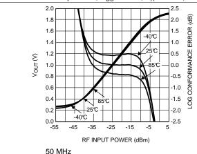
Figure 7. Mean Output Voltage and Log Conformance Error vs RF Input Power
