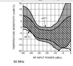
Figure 49. Temperature Sensitivity (Mean ±3 Sigma) vs RF Input Power
