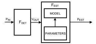
Figure 65. Generic Concept of a Power Measurement System
