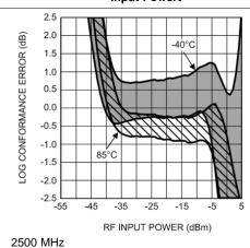
Figure 16. Log Conformance Error (Mean ±3 Sigma) vs RF Input Power
