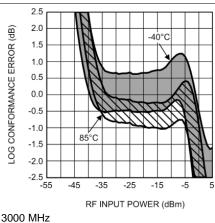
Figure 17. Log Conformance Error (Mean ±3 Sigma) vs RF Input Power
