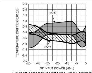
Figure 69. Temperature Drift Error without Temperature Compensation
