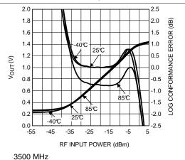
Figure 12. Mean Output Voltage and Log Conformance Error vs RF Input Power
