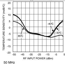
Figure 43. Mean Temperature Sensitivity vs RF Input Power
