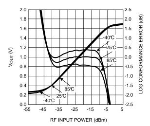
Figure 66. LOG-Conformance Error and LOG-Detector Transfer Function
