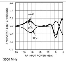
Figure 36. Error For 1-dB Input Power Step vs RF Input Power
