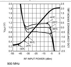
Figure 8. Mean Output Voltage and Log Conformance Error vs RF Input Power
