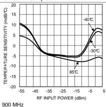
Figure 44. Mean Temperature Sensitivity vs RF Input Power
