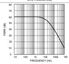
Figure 59. Power Supply Rejection Ratio vs Frequency
