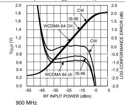
Figure 55. Output Voltage and Log Conformance Error vs RR Input Power for Various Modulation Types
