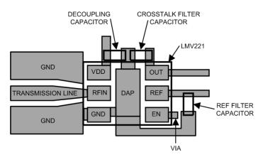
Figure 85. Recommended LMV221 Board Layout
