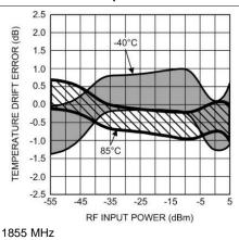
Figure 27. Temperature Drift Error (Mean ±3 Sigma) vs RF Input Power
