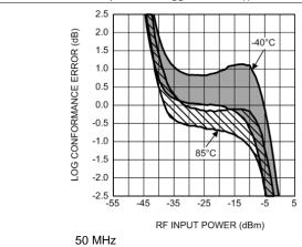
Figure 13. Log Conformance Error (Mean ±3 Sigma) vs RF Input Power
