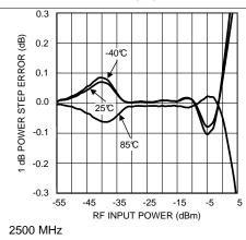
Figure 34. Error For 1-dB Input Power Step vs RF Input
