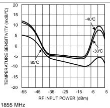
Figure 45. Mean Temperature Sensitivity vs RF Input Power
