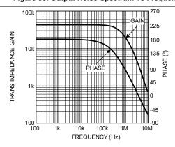
Figure 60. Output Amplifier Gain and Phase vs Frequency
