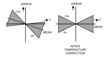
Figure 68. Elimination of the Systematic Component from the Temperature Drift
