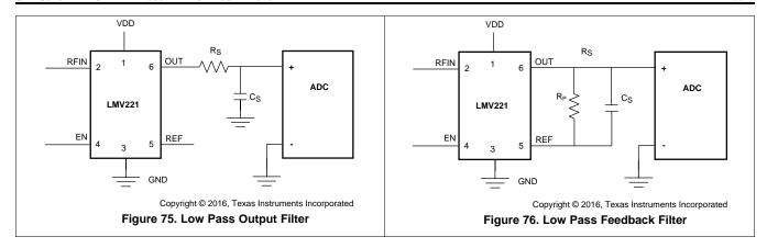
Depending on the system requirements one of the these filtering techniques can be selected. The low pass output filter has the advantage that it preserves the output voltage when the LMV221 is brought into shutdown. This is elaborated in *Output Behavior in Shutdown*. In the feedback filter, resistor R<sub>P</sub> discharges capacitor C<sub>P</sub> in shutdown and therefore changes the output voltage of the device.
