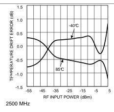
Figure 22. Mean Temperature Drift Error vs RF Input Powert
