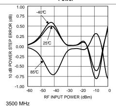
Figure 42. Error For 10-dB Input Power Step vs RF Input Power
