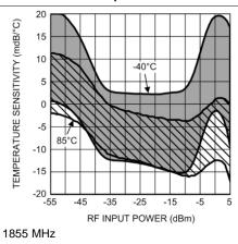
Figure 51. Temperature Sensitivity (Mean ±3 Sigma) vs RF Input Power
