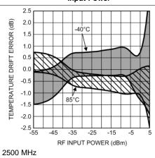
Figure 28. Temperature Drift Error (Mean ±3 Sigma) vs RF Input Power
