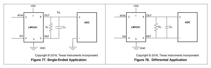
The differential topology has the advantage that it is compensated for temperature drift of the internal reference voltage. This can be explained by looking at the transimpedance amplifier of the LMV221 (Figure 79).
