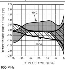
Figure 26. Temperature Drift Error (Mean ±3 Sigma) vs RF Input Power
