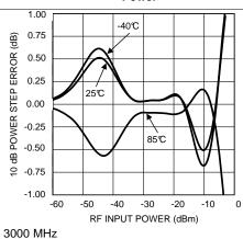
Figure 41. Error For 10-dB Input Power Step vs RF Input
