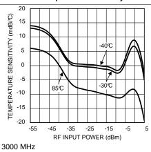
Figure 47. Mean Temperature Sensitivity vs RF Input Power
