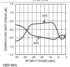
Figure 21. Mean Temperature Drift Error vs RF Input Power
