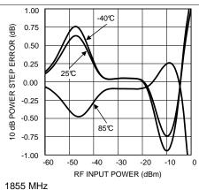
Figure 39. Error For 10-dB Input Power Step vs RF Input Power
