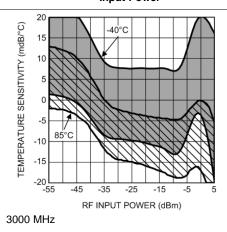
Figure 53. Temperature Sensitivity (Mean ±3 Sigma) vs RF Input Power
