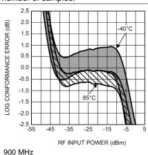
Figure 14. Log Conformance Error (Mean ±3 Sigma) vs RF
