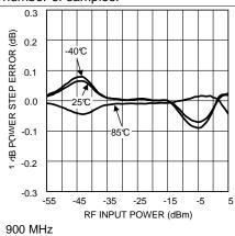
Figure 32. Error For 1-dB Input Power Step vs RF Input
