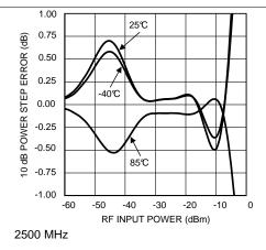
Figure 40. Error For 10-dB Input Power Step vs RF Input Power
