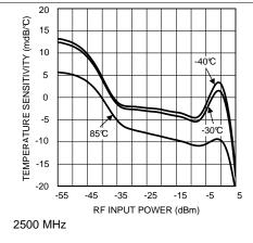
Figure 46. Mean Temperature Sensitivity vs RF Input Power
