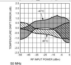
Figure 25. Temperature Drift Error (Mean ±3 Sigma) vs RF Input Power
