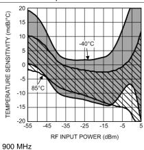
Figure 50. Temperature Sensitivity (Mean ±3 Sigma) vs RF Input Power
