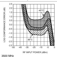
Figure 18. Log Conformance Error (Mean ±3 Sigma) vs RF Input Power
