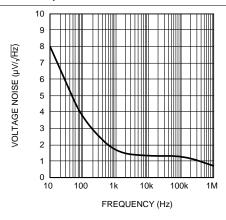
Figure 58. Output Noise Spectrum vs Frequency
