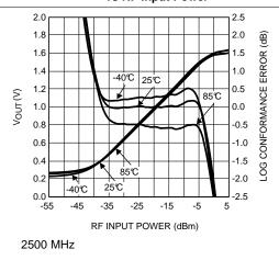
Figure 10. Mean Output Voltage and Log Conformance Error vs RF Input Power
