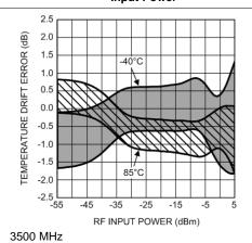
Figure 30. Temperature Drift Error (Mean ±3 Sigma) vs RF Input Power
