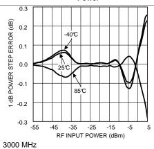
Figure 35. Error For 1-dB Input Power Step vs RFInput Power
