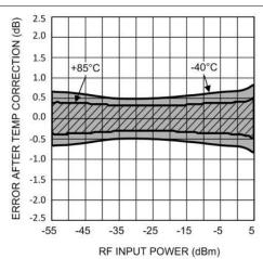
Figure 70. Temperature Drift Error With Temperature Compensation
