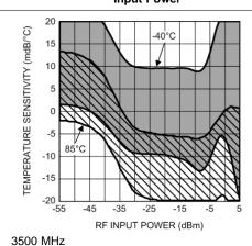
Figure 54. Temperature Sensitivity (Mean ±3 Sigma) vs RF Input Power
