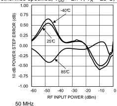
Figure 37. Error For 10-dB Input Power Step vs RF Input Power
