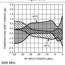
Figure 29. Temperature Drift Error (Mean ±3 Sigma) vs RF Input Power
