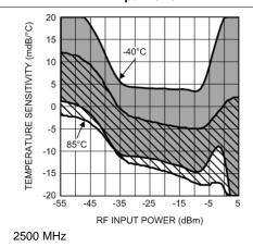
Figure 52. Temperature Sensitivity (Mean ±3 Sigma) vs RF Input Power
