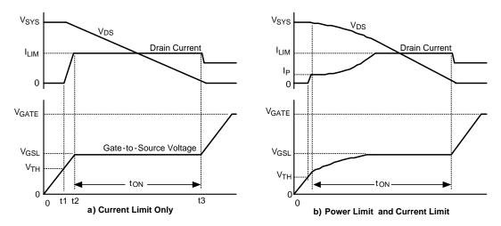
Figure 30. MOSFET Power Up Waveforms
