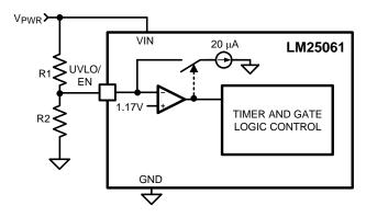
Figure 31. Programming the UVLO Thresholds
