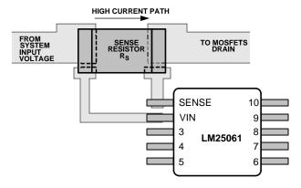
Figure 27. Sense Resistor Connections
