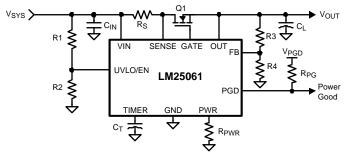
Figure 21. Basic Application Circuit
