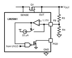
Figure 33. Programming the PGD Threshold
