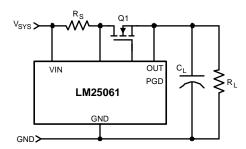
Figure 29. Load Draws Current During Turn-On
