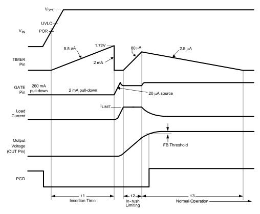
Figure 23. Power Up Sequence (Current Limit only)
