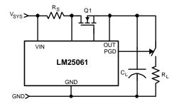
Figure 28. No Load Current During Turn-On
