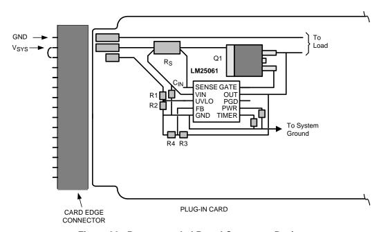
Figure 36. Recommended Board Connector Design
