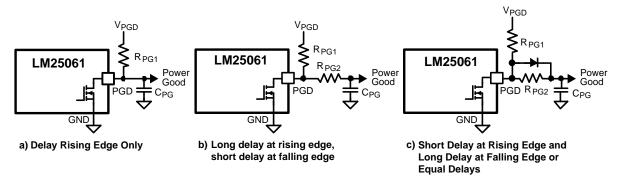
Figure 35. Adding Delay to the Power Good Output Pin
