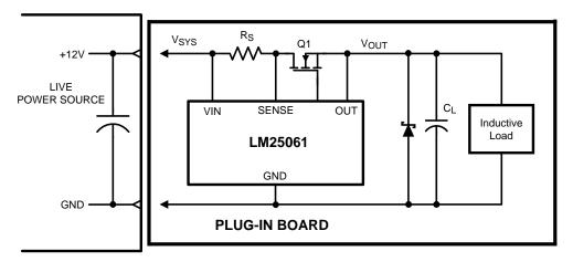
Figure 37. Output Diode Required for Inductive Loads
