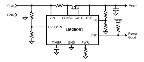
Figure 1. Positive Power Supply Control
