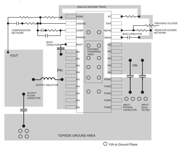
Figure 9. TPS54972 PCB Layout
