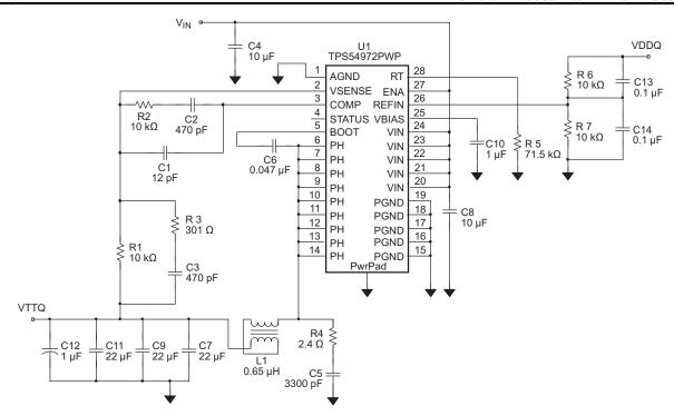
Figure 8. Application Circuit
