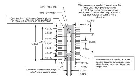
Figure 10. Recommended Land Pattern for 28-Pin PWP PowerPAD
