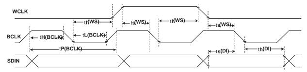
Figure 4. DSP Timing in Slave Mode
