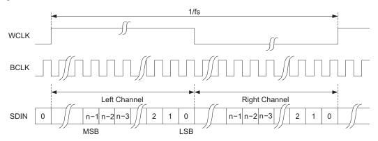
Figure 26. Right Justified Serial Bus Mode Operation
