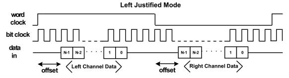
Figure 30. DSP Mode and Left Justified Modes, Showing the Effect of a Programmed Data Word Offset
