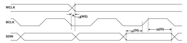
Figure 1. I<sup>2</sup>S/LJF/RJF Timing in Master Mode
