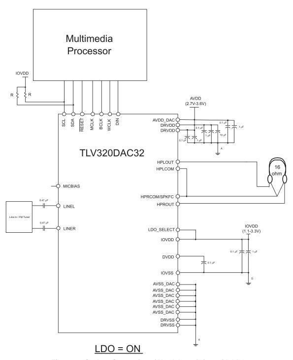
Figure 17. Capless Connection of Headphone Driver with LDO
