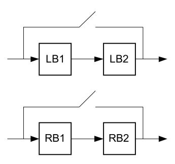
Figure 32. Structure of the Digital Effects Processing for Independent Channel Processing
