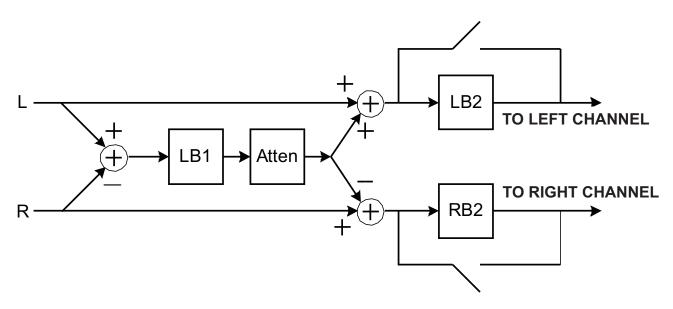
Figure 33. Architecture of the Digital Audio Processing When 3-D Effects are Enabled
