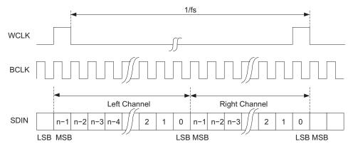
Figure 29. DSP Serial Bus Mode Operation
