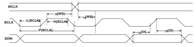
Figure 3. I<sup>2</sup>S/LJF/RJF Timing in Slave Mode
