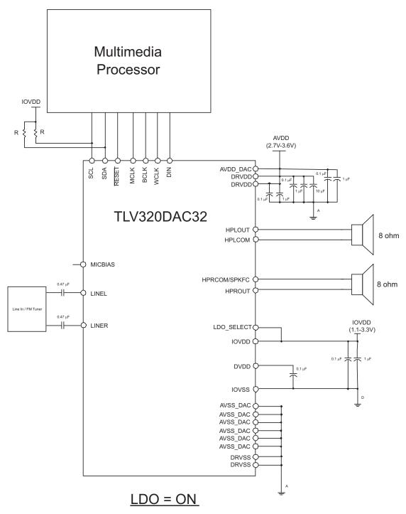
Figure 15. Internal 8-Ω Speaker Driver with LDO
