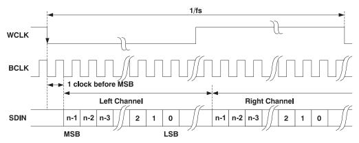
Figure 28. I<sup>2</sup>S Serial Data Bus Mode Operation
