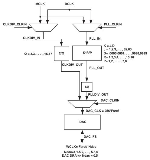
Figure 31. Audio Clock Generation Processing
