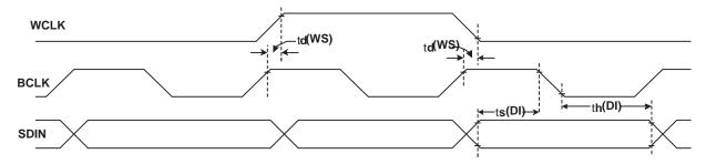
Figure 2. DSP Timing in Master Mode
