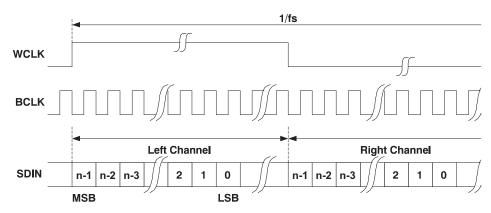
Figure 27. Left Justified Serial Data Bus Mode Operation
