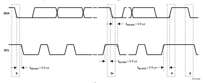
Figure 23. I<sup>2</sup>C Interface Timing
