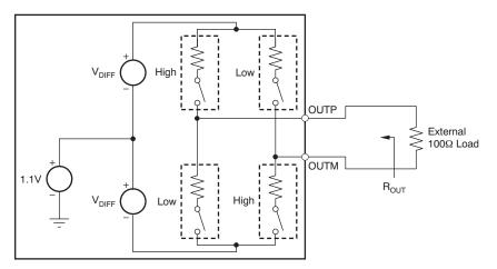
NOTE: Use the default buffer strength to match  $100-\Omega$  external termination (R<sub>OUT</sub> =  $100 \Omega$ ). To match with a  $50-\Omega$  external termination, set the LVDS STRENGTH bit (R<sub>OUT</sub> =  $50 \Omega$ ).
