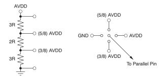
Figure 65. Simplified Diagram to Configure the DFS Pin
