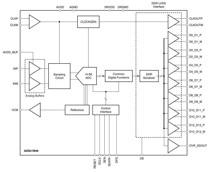
Figure 53. ADS41B49 Block Diagram
