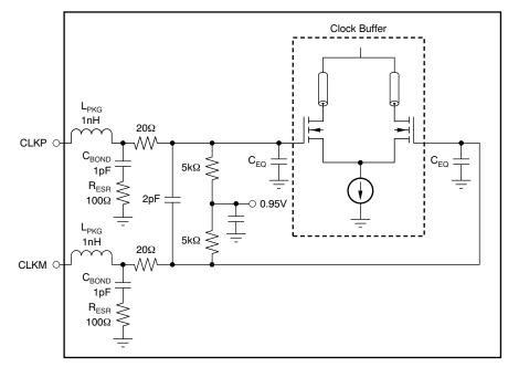
NOTE: C<sub>EQ</sub> is 1 pF to 3 pF and is the equivalent input capacitance of the clock buffer.
