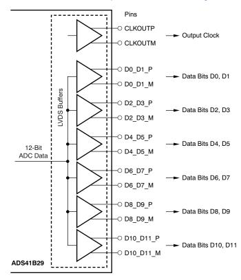
Figure 59. ADS41B29 LVDS Data Outputs
