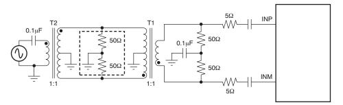
Figure 86. Drive Circuit for High Input Frequencies
