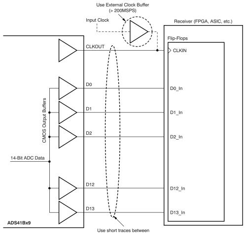
ADC output and receiver pins (1 to 2 inches).
