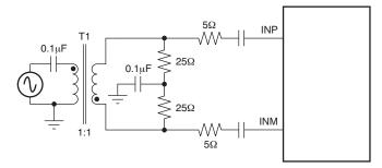
Figure 85. Drive Circuit for Low Input Frequencies
