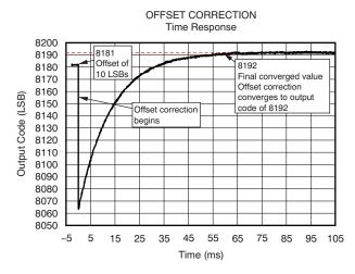
Figure 58. Time Response of Offset Correction
