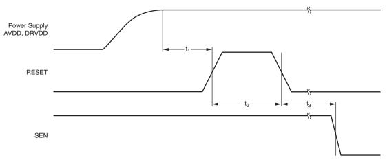
NOTE: A high pulse on the RESET pin is required in the serial interface mode in case of initialization through hardware reset. For parallel interface operation, RESET must be permanently tied high.
