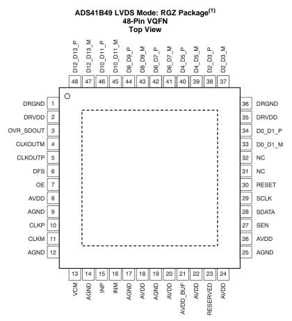
(1) The PowerPAD<sup>™</sup> is connected to DRGND.
