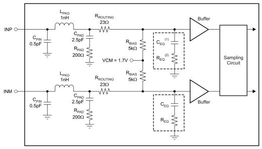
(1)  $C_{EQ}$  refers to the equivalent input capacitance of the buffer = 4 pF.
