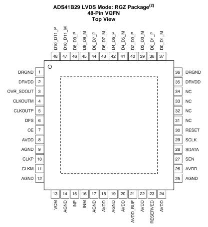
(1) The PowerPAD is connected to DRGND.
