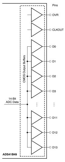
Figure 63. CMOS Output Interface
