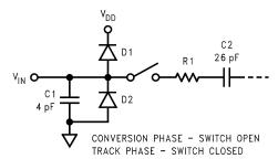
Figure 31. Equivalent Input Circuit
