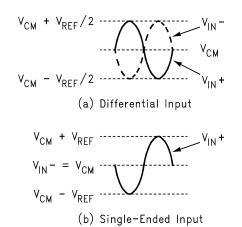
Figure 18. Expected Input Signal Range
