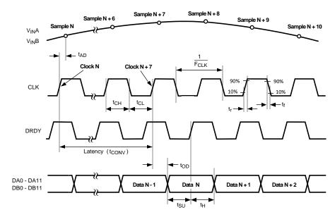
Figure 2. Output Timing
