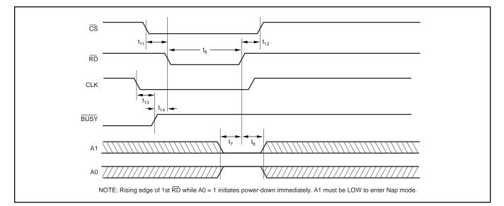
FIGURE 3. Entering Nap Using RD and A0.
