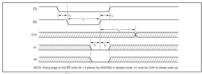
FIGURE 4. Initiating Wake-Up Using RD and A0.
