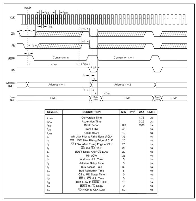
FIGURE 2. ADS7852 Write/Read Timing.
