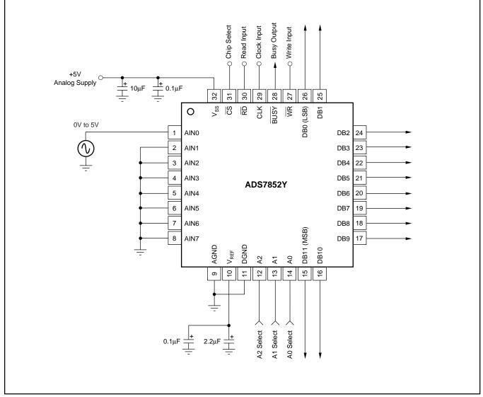
FIGURE 1. Typical Circuit Configuration.
