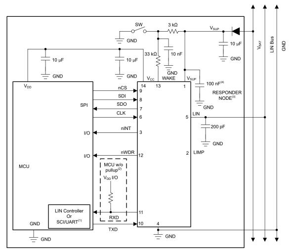
If RXD on MCU or LIN responder has internal pullup; no external pullup resistor is needed.
