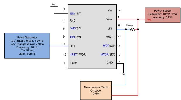
图 8-6. Test Circuit for I<sub>BUS\_LIM</sub> at Dominant State (Driver on)
