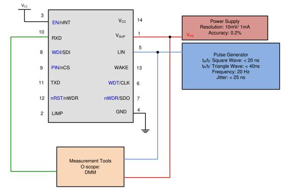
图 8-4. LIN Receiver Test with RX access
