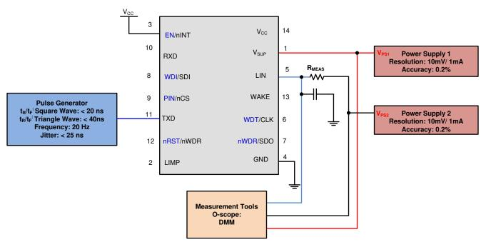
图 8-11. Test Circuit Slope Control and Duty Cycle
