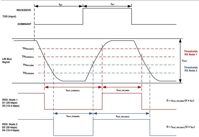
图 8-12. Definition of Bus Timing
