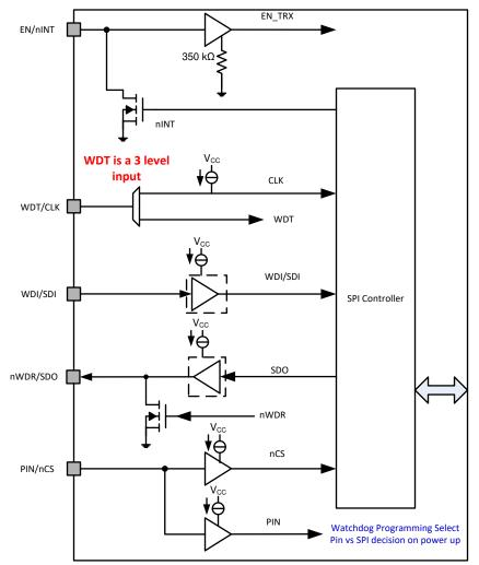
图 9-2. Input and Output High Level Functional Block Diagram
