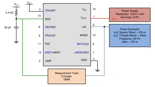
图 8-13. Propagation Delay Test Circuit
