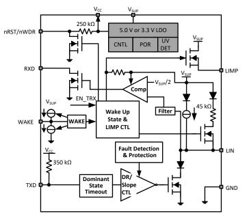
图 9-1. Transceiver plus VREG Functional Block Diagram
