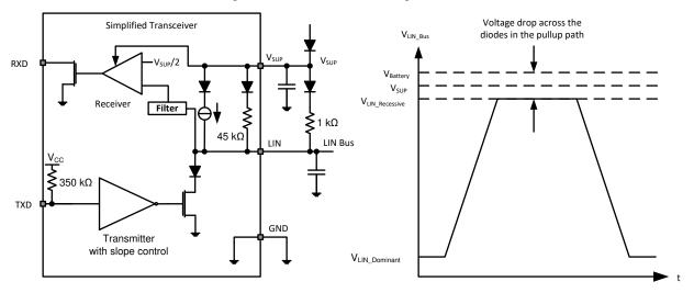
图 9-3. Commander Node Configuration with Voltage Levels
