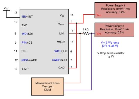
图 8-9. Test Circuit for I<sub>BUS\_NO\_GND</sub> Loss of GND
