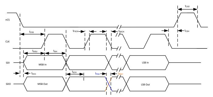
图 8-18. SPI AC Characteristic for Read and Write
