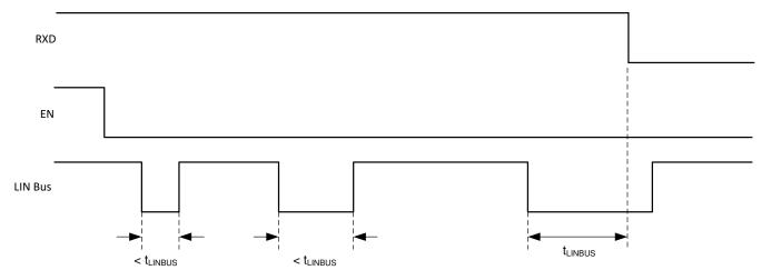
图 9-5. No Bus Fault: Entering Sleep Mode with Bus Recessive Condition and Wakeup
