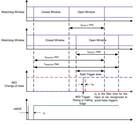
图 8-19. Watchdog Window Timing Diagram
