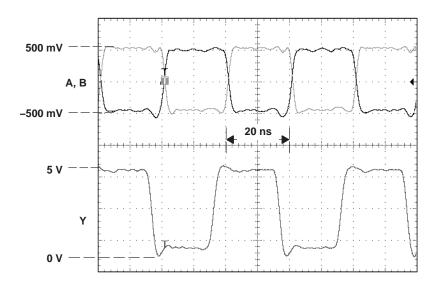
Figure 10. Receiver Inputs and Outputs, 50 Mbps Signaling Rate
