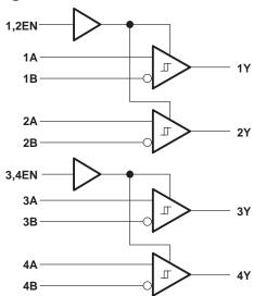
Each receiver operates over a wide range of positive and negative common-mode input voltages, and features ESD protection to 6 kV, making it suitable for high-speed multipoint data transmission applications in harsh environments. These devices are designed using LinBiCMOS™, facilitating low power consumption and inherent robustness.
