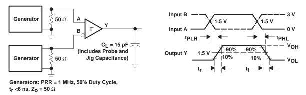
Figure 2. Switching Test Circuit and Waveforms
