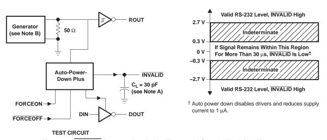
Figure 4. INVALID Propagation Delay Times and Supply Enabling Time
