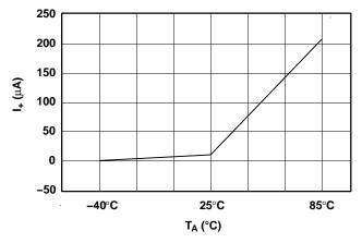
Figure 13. Power-Supply Current vs Temperature (V<sub>+</sub> = 5 V)
