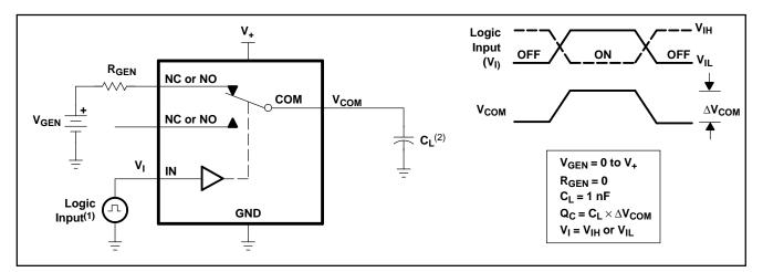
A. C<sub>1</sub> includes probe and jig capacitance.
