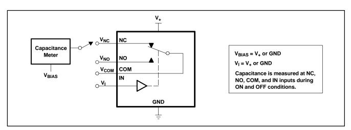
Figure 17. Capacitance (C<sub>1</sub>, C<sub>COM(ON)</sub>, C<sub>NC(OFF)</sub>, C<sub>NO(OFF)</sub>, C<sub>NC(ON)</sub>, C<sub>NO(ON)</sub>)
