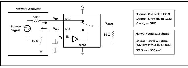
A. All input pulses are supplied by generators having the following characteristics: PRR  $\leq$  10 MHz, Z<sub>O</sub> = 50  $\Omega$ , t<sub>r</sub> < 5 ns, t<sub>f</sub> < 5 ns.
