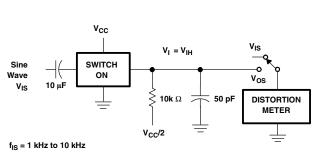
**Figure 5. Sine-Wave Distortion Test Circuit**
