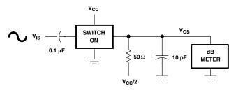
Figure 3. Frequency-Response Test Circuit
