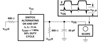
Figure 6. Control-to-Switch Feedthrough Noise Test Circuit
