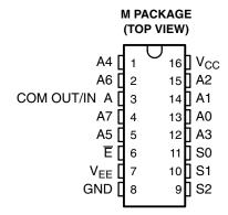
This analog multiplexer/demultiplexer controls analog voltages that may vary across the voltage supply range (i.e.,  $V_{CC}$  to  $V_{EE}$ ). It is a bidirectional switch that allows any analog input to be used as an output and vice-versa. The switch has low ON resistance and low OFF leakages. In addition, this device has an enable control that, when high, disables all switches to their OFF state.
