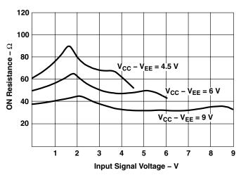
Figure 9. Typical ON Resistance vs Input Signal Voltage
