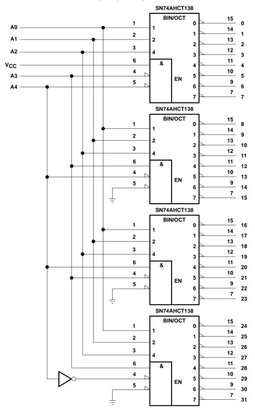
Figure 3. 32-Bit Decoding Scheme
