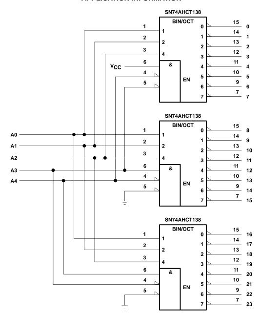
Figure 2. 24-Bit Decoding Scheme
