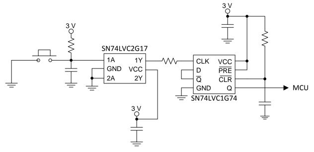
Figure 4. Device Power Button Circuit
