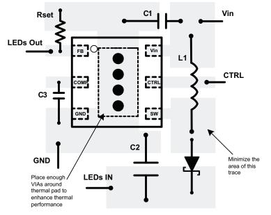
Figure 19. TPS61161-Q1 Layout Example
