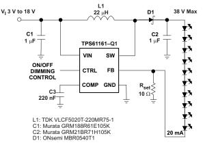
Figure 15. LED Drivers With 10 White LEDs Schematic
