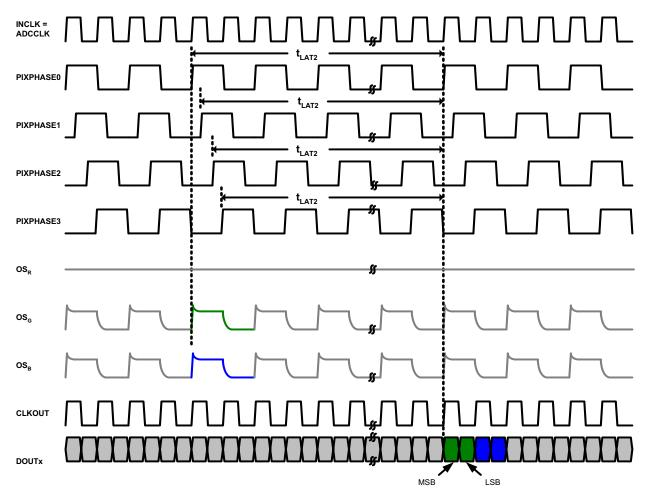
Data latency shown is for Mode 2 in relation to PIXPHASE0 with the processing order set to  $OS_a = OS_B$ . If the incoming pixels are not aligned with PIXPHASE0, one of the remaining PIXPHASEs can be selected as the sampling phase without effecting the output data location.
