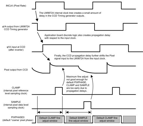
Figure 23. CCD Output Phase Shift in a Real Application
