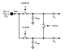
Figure 14. CDS Mode Input Bias Current
