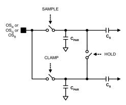
Figure 13. CDS Mode Simplified Input Diagram
