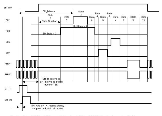
Signal levels in each SH Interval State are set by the settings "SH State x LSPIX 12-0" settings in pages 4 and 5 of the register table. The SH State settings are 1 = high. These internal signals can be inverted by the polarity settings for each signal output found in Page 7.
