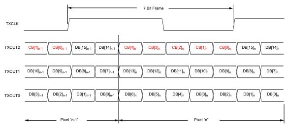
Figure 49. LVDS Output Bit Alignment and Data Format
