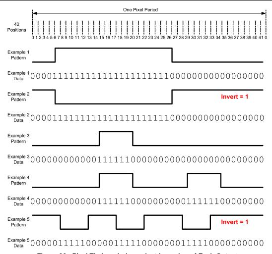
Figure 36. Pixel Timing - Independent Inversion of Each Output
