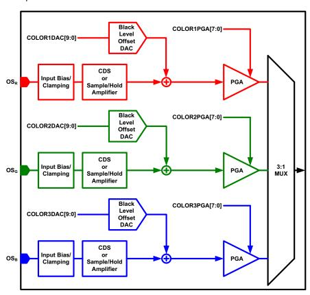
Figure 6. Synchronous Three Channel Pixel Mode Signal Routing
