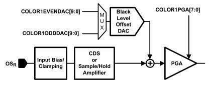
Figure 15. Analog Offset Applied Prior to POA
