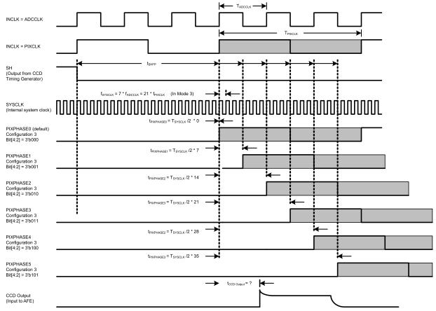
The CCD output will usually have a measurable delay with respect to the input clock to the AFE. The AFE's internal sampling clocks are based on one of six PIXPHASE clocks. These PIXPHASE settings provide coarse adjustment of the internal AFE clock domain to best match the phase of the incoming CCD signal. Fine adjustment of the sampling clocks is discussed in another section. In this example above, PIXPHASE2 appears to provide the closest match for the incoming CCD signal.
