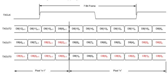
Figure 50. LVDS Output Bit Alignment and Data Format
