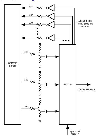
Figure 21. Typical AFE/CCD Interface
