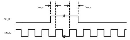
Figure 44. SH\_R to INCLK (PIXCLK or ADCCLK) Timing
