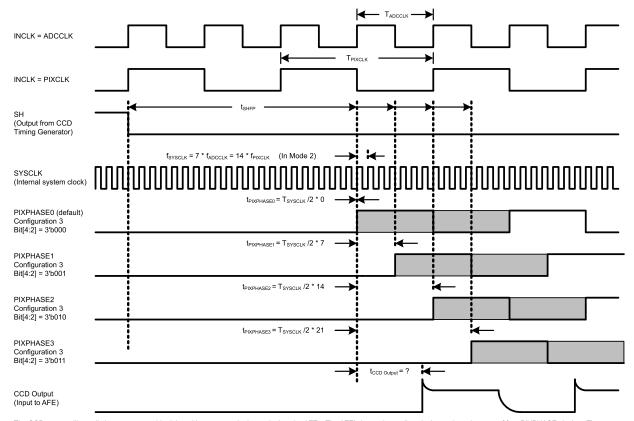
The CCD output will usually have a measurable delay with respect to the input clock to the AFE . The AFE's internal sampling clocks are based on one of four PIXPHASE clocks . These PIXPHASE settings provide coarse adjustment of the internal AFE clock domain to best match the phase of the incoming CCD signal . Fine adjustment of the sampling clocks is discussed in another section. In this example above, PIXPHASE2 appears to provide the closest match for the incoming CCD signal .
