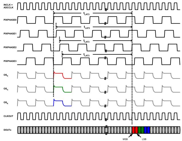
Data latency shown is for Mode 3 in relation to PIXPHASE0 with the processing order set to  $OS_R = OS_B = OS_B$ . If the incoming pixels are not aligned with PIXPHASE0, one of the remaining PIXPHASEs can be selected as the sampling phase without effecting the output data location.
