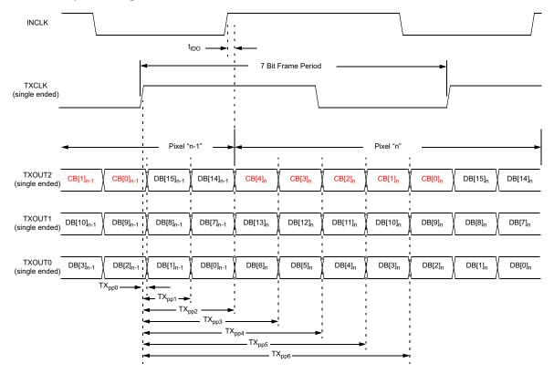
Figure 53. LVDS Data Output Mode Specification Diagram
