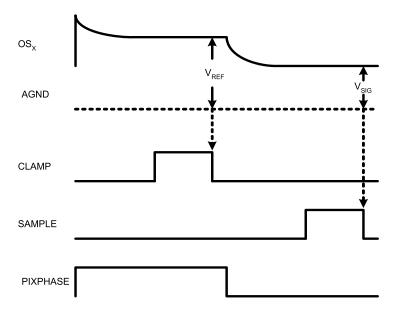
CLAMP and SAMPLE are the internal sampling clocks for the input CDS amplifier. CLAMP and SAMPLE are adjustable within the selected PIXPHASE
