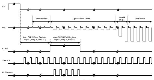
Figure 10. Typical CCD Waveform and LM98725 Input Clamp Signal (CLPIN)
