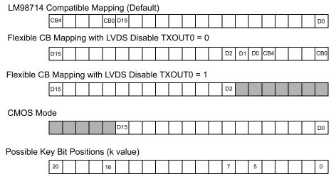
(1) If an output bit is replaced with the scrambler key, that bit position/value is excluded from the calculation of the parity.
