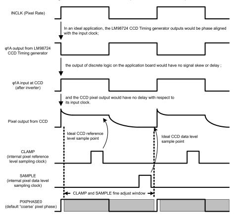
By default, the LM98724's internal sampling clocks (CLAMP and SAMPLE) are adjustable within PIXPHASE0, an internal pixel rate clock which is in phase with the input clock.
