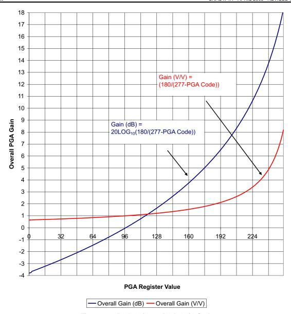
Figure 18. PGA Gain vs. PGA Gain Code
