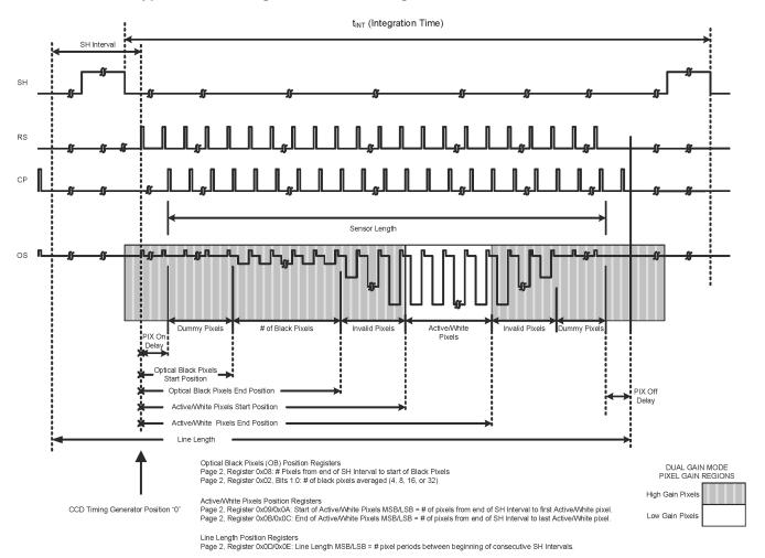
Figure 19. Typical Line Timing and Pixel Gain Regions
