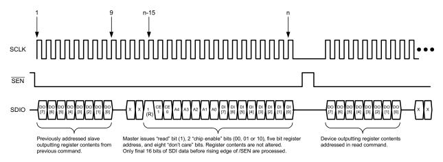
Figure 63. Serial Read - LM98714 Compatible Connection
