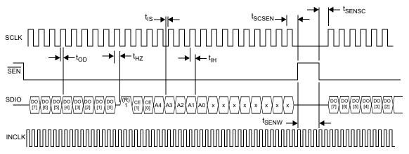
Figure 1. Serial Interface Specification Diagram
