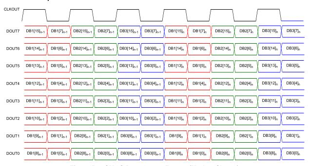
Figure 58. CMOS Data Output Format (Mode 3 Shown)
