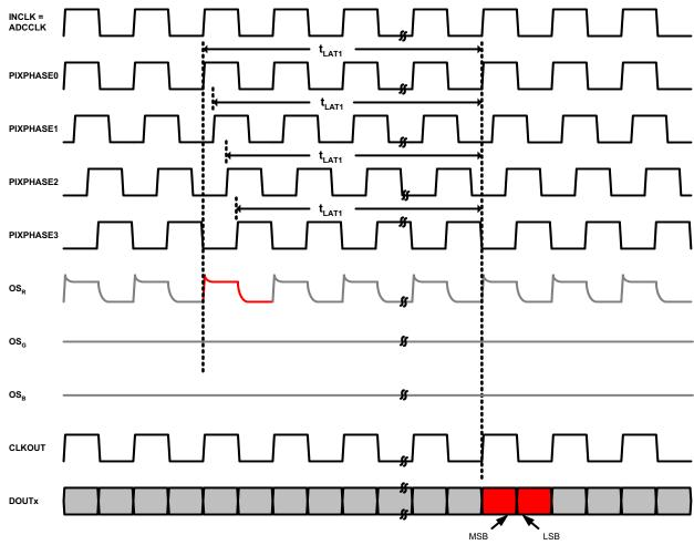
Data latency shown is for Mode 1 in relation to PIXPHASE0 with the processing channel configured to OS<sub>R</sub>. If the incoming pixels are not aligned with PIXPHASE0, one of the remaining PIXPHASEs can be selected as the sampling phase without effecting the output data location.
