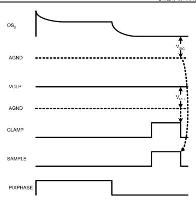
CLAMP and SAMPLE are the internal sampling clocks for the input CDS amplifier. CLAMP and SAMPLE are adjustable within the selected PIXPHASE setting.
