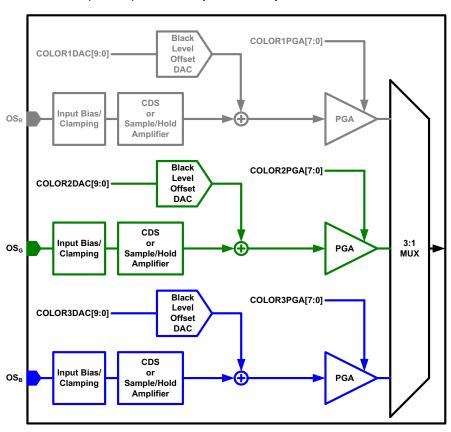
Figure 7. Mode 2 Signal Routing
