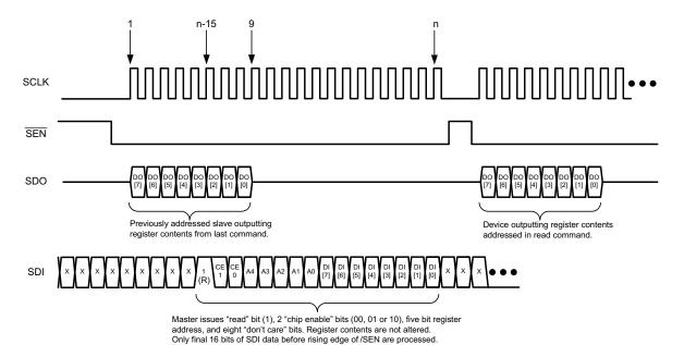
Figure 67. Serial Read - 4 Wire Connection - 16+ Clock Mode
