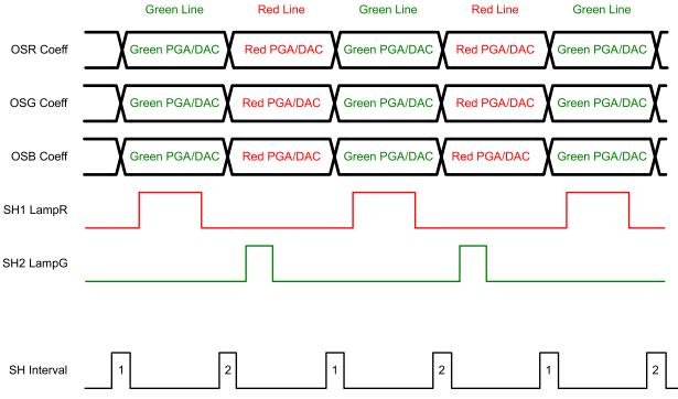
Use Page 2, Register 10h, Bits 6:5 to choose which SHx Lampx outputs are used, and which coefficients are used in CISb 2 color sequence.
