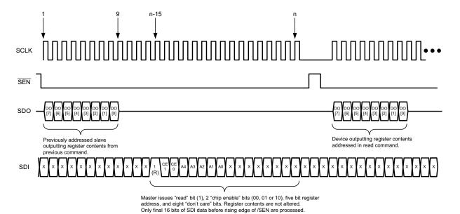
Figure 65. Serial Read - 4 Wire Connection - 25+ Clock Mode
