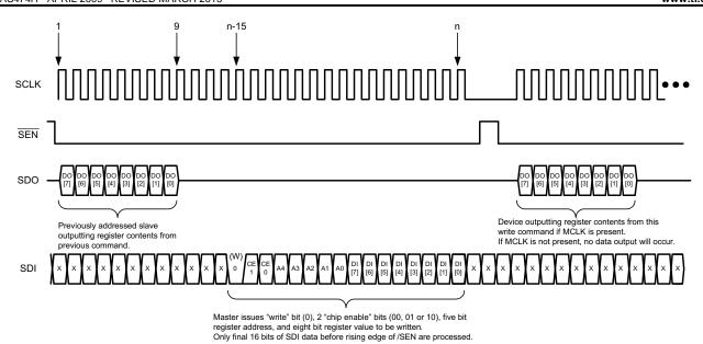
Figure 64. Serial Write - 4 Wire Connection - 25+ Clock Mode
