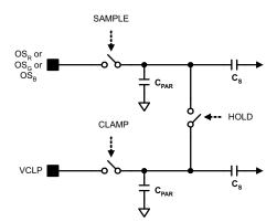
Figure 11. Sample and Hold Mode Simplified Input Diagram
