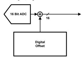
Figure 16. Digital Offset Applied to ADC Output
