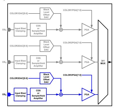
Figure 8. Mode 1a Signal Routing
