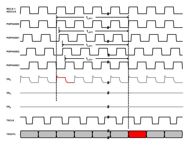
Data latency shown is for Mode 1 in relation to PIXPHASE0 with the processing channel configured to  $OS_R$ . If the incoming pixels are not aligned with PIXPHASE0, one of the remaining PIXPHASEs can be selected as the sampling phase without effecting the output data location.
