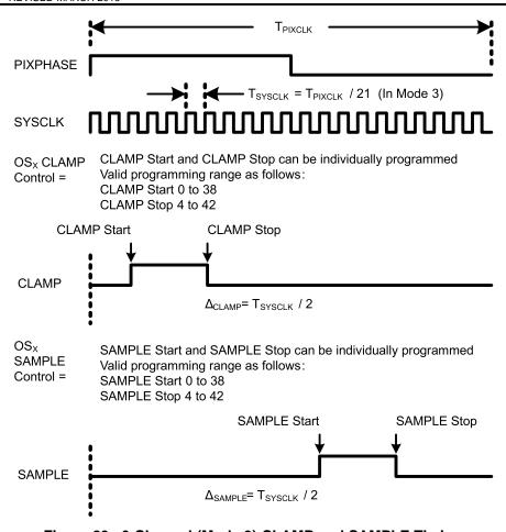
Figure 29. 3 Channel (Mode 3) CLAMP and SAMPLE Timing
