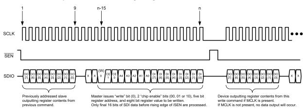
Figure 62. Serial Write - LM98714 Compatible Connection
