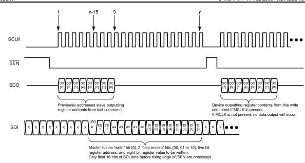
Figure 66. Serial Write - 4 Wire Connection - 16+ Clock Mode
