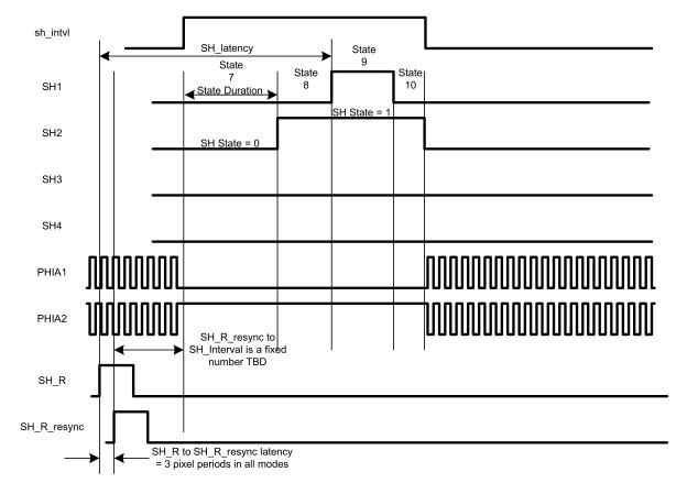
In the Second SH Interval, SH States 7 to 14 are available. The SH interval ends at the first zero length SH State. In this example, only states 7, 8, 9, 10 are used.
