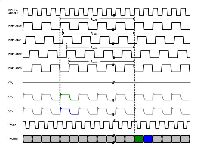
Data latency shown is for Mode 2 in relation to PIXPHASE0 with the processing order set to  $OS_q \\cdot OS_g$ . If the incoming pixels are not aligned with PIXPHASE0, one of the remaining PIXPHASEs can be selected as the sampling phase without effecting the output data location.
