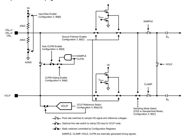
Figure 9. Input Bias and Clamping Diagram
