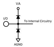
Figure 2. Analog Input Protection
