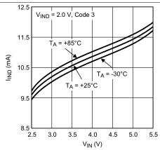
Figure 16. Indicator Current vs Input Voltage Tri-Temp
