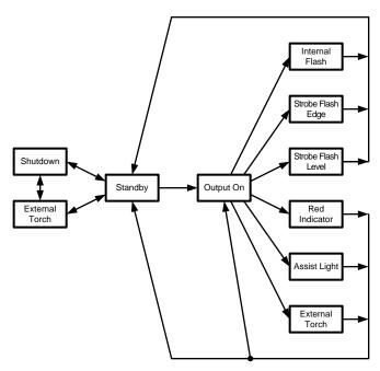
Figure 40. I<sup>2</sup>C Control State Diagram
