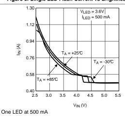
Figure 11. Input Current vs Input Voltage
