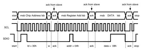
w = write (SDA = 0); ack = acknowledge (SDA pulled down by the slave): id = chip address, 30h for LM3555
