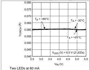
Figure 7. Torch Current vs Input Voltage
