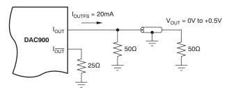
Figure 6. Driving a Doubly-Terminated 50Ω Cable Directly
