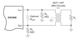
Figure 3. Differential Output Configuration Using an RF Transformer
