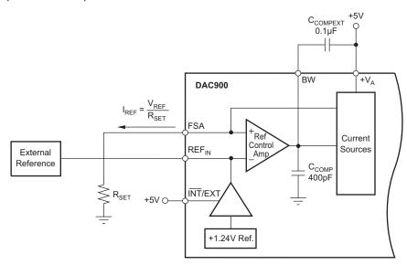
Figure 8. External Reference Configuration
