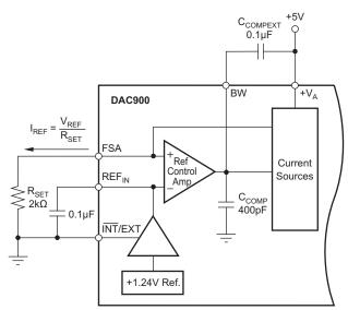
Figure 7. Internal Reference Configuration
