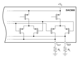
Figure 2. Equivalent Analog Output
