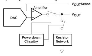
Figure 31. Output Stage During Power Down (High-Impedance)
