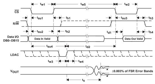
Figure 1. Data Read/Write Timing
