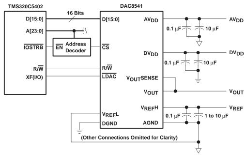
Figure 33. DAC8541 to TMS320 DSP
