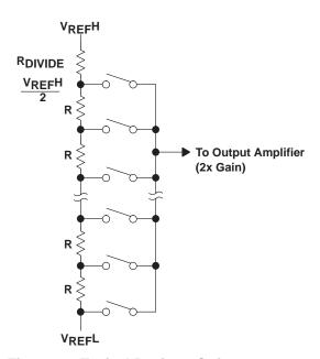
Figure 30. Typical Resistor String
