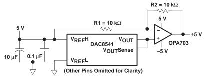
Figure 34. Bipolar Operation With the DAC8541
