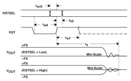
Figure 2. Reset Timing
