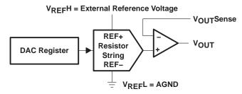
Figure 29. Generalized DAC Architecture
